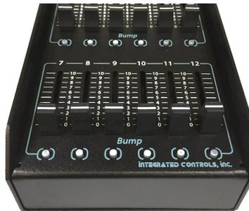
Don't let the name -12 worry you, the full 512 channels of starting address are available by setting a DIP switch on the rear panel.
