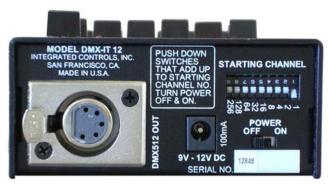
Unit is shown as shipped with starting channel set to 1
